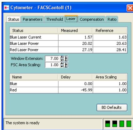
Values entered in the Laser tab apply globally to BD FACSDiva software. They are not saved with experiments or tubes. The values at startup are the last entered values.
