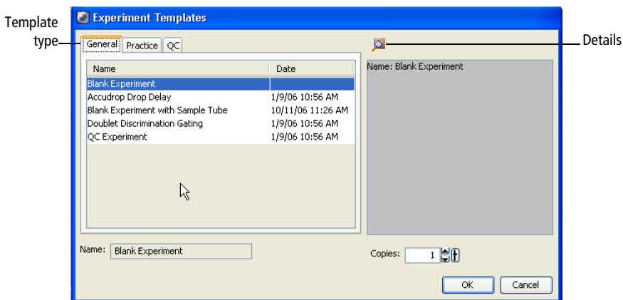
To view the experiment layout associated with the experiment template, click the **Details** button. The Experiment Layout opens, showing the specimens and tubes in the experiment, and any defined labels, keywords, and acquisition criteria. See Using the Experiment Layout on page 60.
