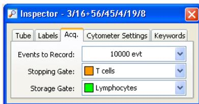
The cytometer would keep acquiring until 10,000 events were collected in the T cell gate. However, only events that fell into the Lymphocytes gate would be saved to the database.
