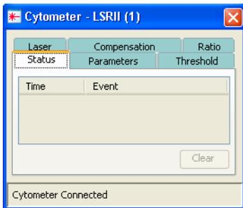
If the Status tab is hidden by another tab, it turns red to alert you when a message is sent from the cytometer. If the Status tab or Cytometer window is hidden when a message is sent, the window icon appears at the top of the workspace with a message alerting you to check the Status tab.
