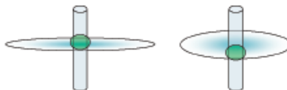
Figure 1b. With a 12-micron particle, however, the BD FACSAria acts more as a slit-scanning cytometer because the cell is larger than the beam height.
