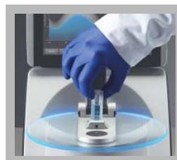
**Measure using a Cuvette**
