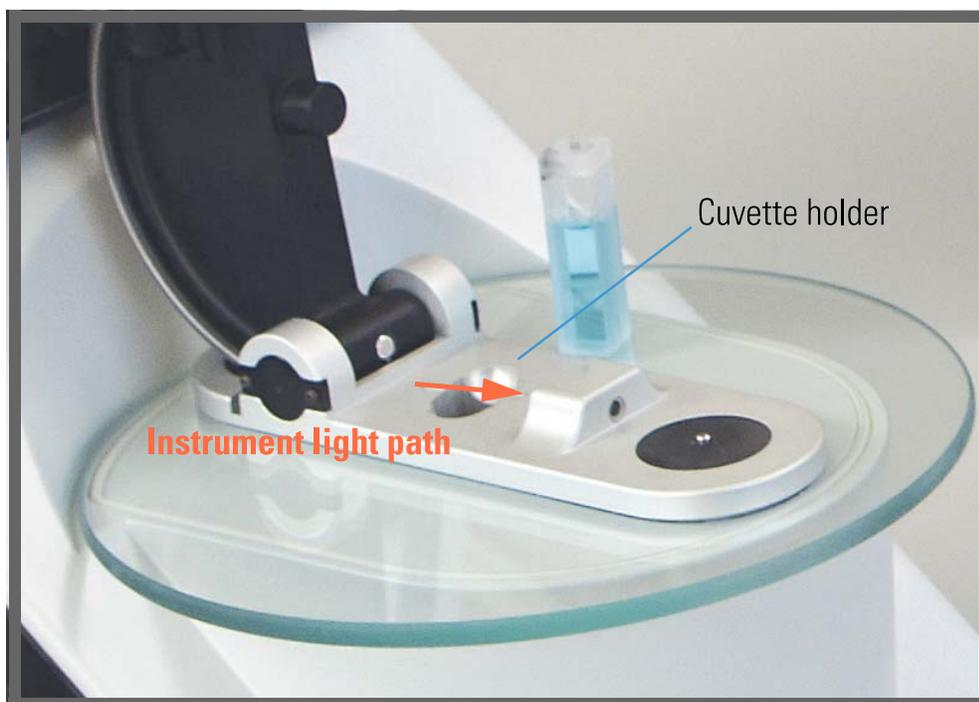
The NanoDrop One<sup>C</sup> model includes a cuvette holder for measuring dilute samples, colorimetric assays, cell cultures and kinetic studies. The cuvette system has these additional features:
