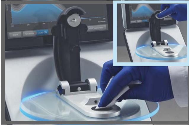
3. Lift the instrument arm and clean the upper and lower pedestals with new laboratory wipe.
