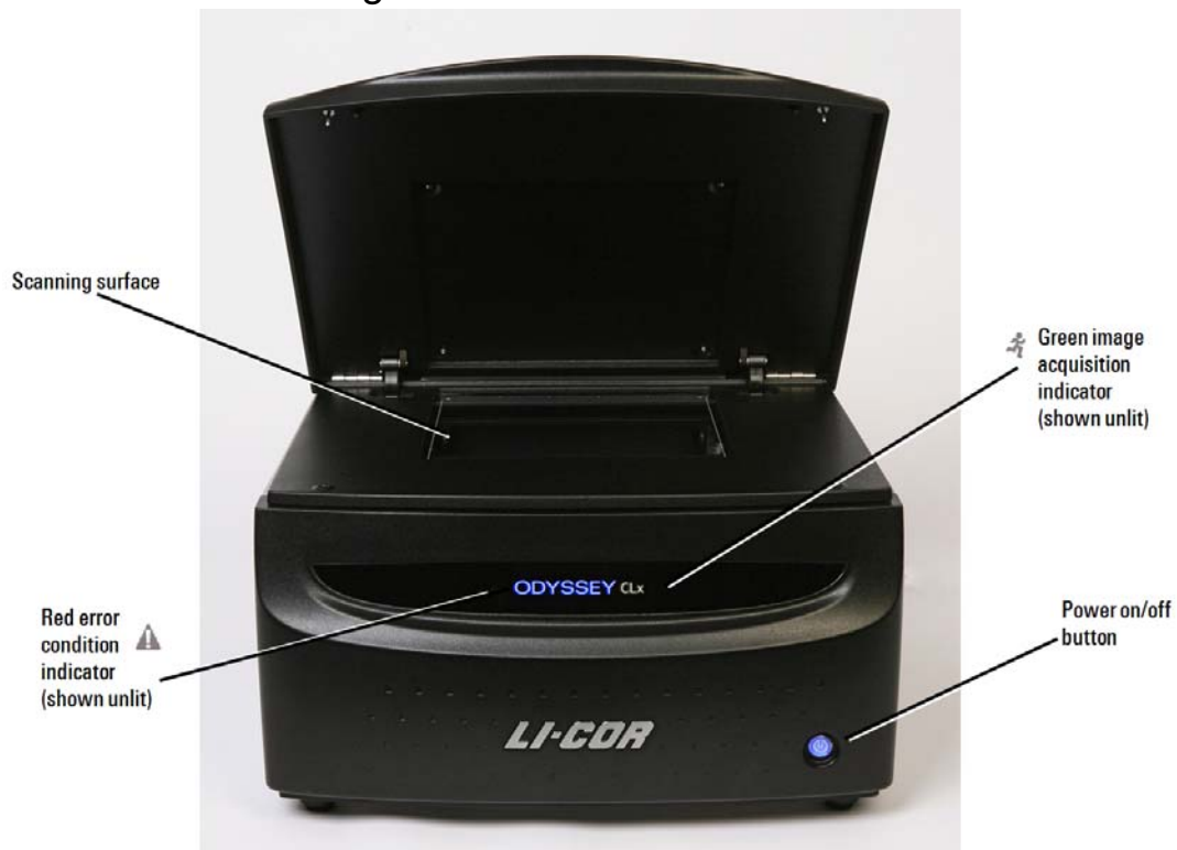
Figure 2-1. Front panel features and power button on the Odyssey CLx Imager.
