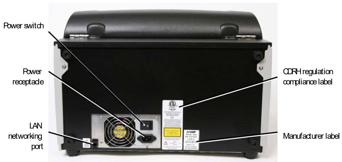
Figure 2-3. Closeup of the Odyssey®CLx Imager rear panel showing the power receptacle and LAN port (use only the supplied networking cable). Also shown are the CDRH regulation compliance label, the manufacturer label and the power switch. The power switch can be left in the 'on' position. Note: The appearance of your instrument's back panel may vary slightly from the one shown.
