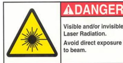
The following laser warning label appears on the interior side panels near release mechanisms and next to hood latch release.
